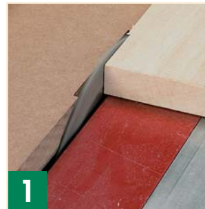
▲ The recessed infeed edge of the fence guides the workpiece into the blade.
