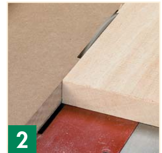
▲ The full-width, outfeed portion of the fence supports the jointed edge.
